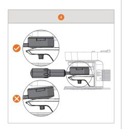
**10.** Make sure the port-a-filter does not wiggle after adjusting. **4**
